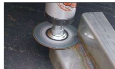
Thin cutting disc Safecut DC: 75x1,0x9,52 A60SX
