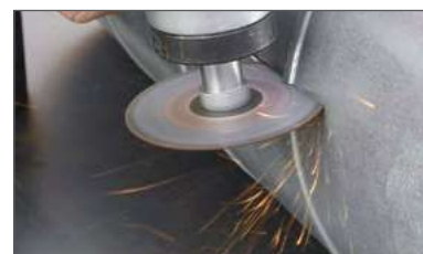
Thin cutting disc ZIP HP: 75x1,0x9,52 A60SX
