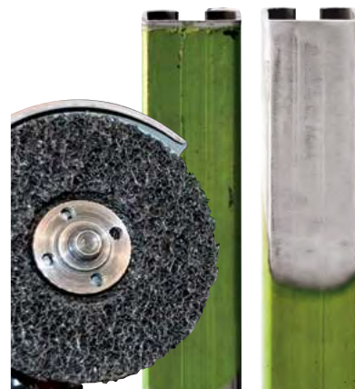
Before and after SCRUBBER pass on a stove enamelled tube.
